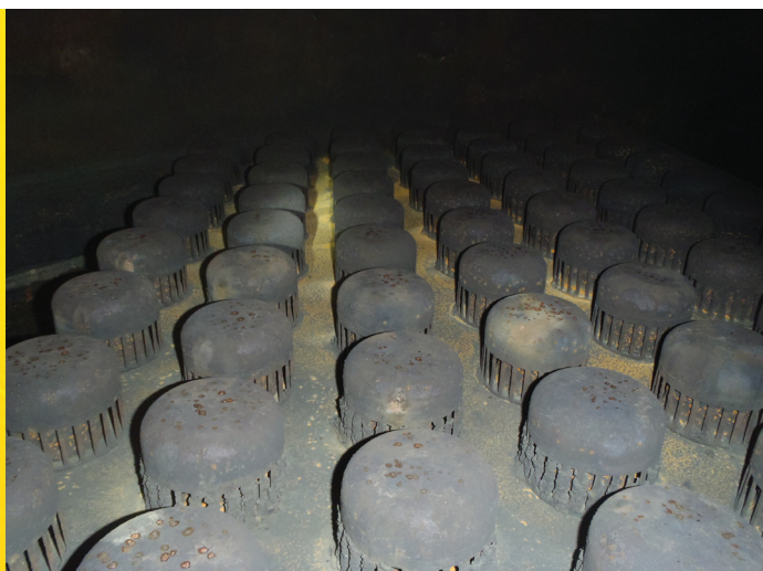
Tower Bubble Caps Following Treatment
