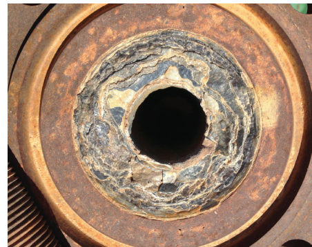
Piping contaminated with NORM
