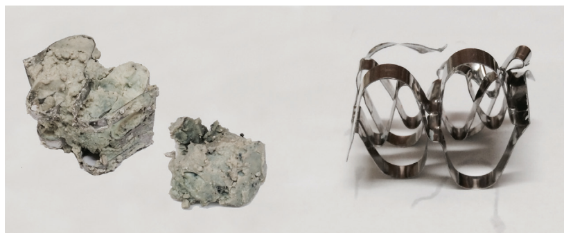
Chemically Cleaned Raschig Ring - 10% FQE Dithiazine Clean - 65°C (150°F), 4 hours
