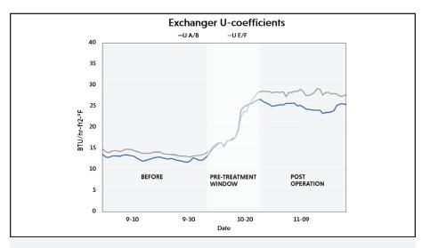
The graph above (provided by the client) shows the effectiveness of FQE Solvent-H+ at increasing the efficiency of the online crude unit heat exchangers.
