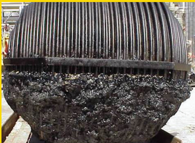
Propane deasphalter heat exchanger bundle following competitive cleaning process .
